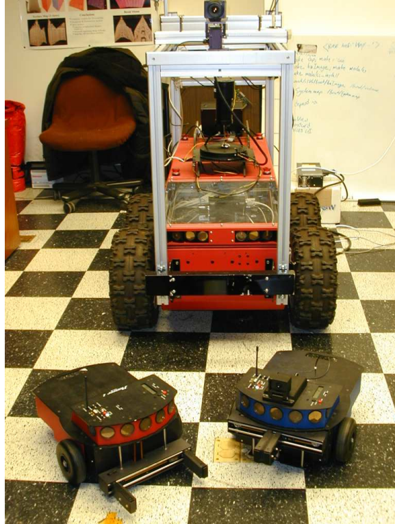
Figure 1: Our three RWII/Mobility-compatible robots. The large robot in the middle/back is our ATRV2 annotated in detail in figure 2. The smaller robots in the foreground are a pair of Pioneer1's.
